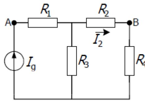
$$I_2 = \frac{R_3 + R_4}{R_2 + R_3 + R_4} I_g = \frac{15 \Omega}{25 \Omega} \cdot 2,6 \text{ A} = 1,56 \text{ A}$$
