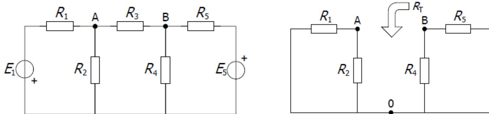
$$R_T = (R_1 \parallel R_2) + (R_4 \parallel R_5) = \frac{R_1 R_2}{R_1 + R_2} + \frac{R_4 R_5}{R_4 + R_5} = 1,9 \Omega + 10 \Omega = 11,9 \Omega$$
