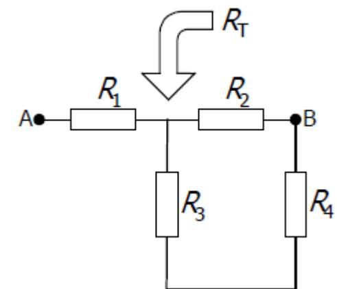
$$R_T = (R_3 + R_4) \parallel R_2 + R_1 = \frac{(R_3 + R_4)R_2}{R_3 + R_4 + R_2} + R_1 = 26 \Omega$$
