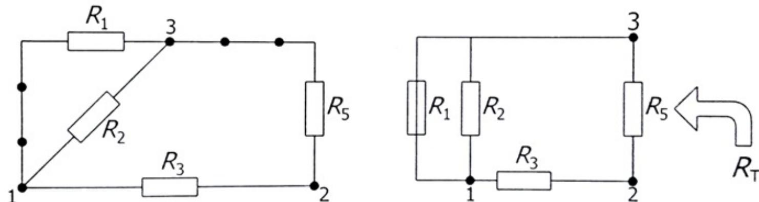
$$R_T = ((R_1 || R_2) + R_3) || R_5 = \frac{\left( \frac{R_1 R_2}{R_1 + R_2} + R_3 \right) R_5}{\frac{R_1 R_2}{R_1 + R_2} + R_3 + R_5} = 562.5\Omega$$
