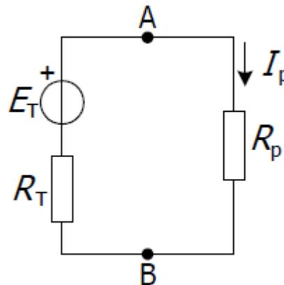
$$I_p = \frac{E_T}{R_T + R_p} = \frac{67,6 \text{ V}}{52 \Omega} = 1,3 \text{ A}$$
