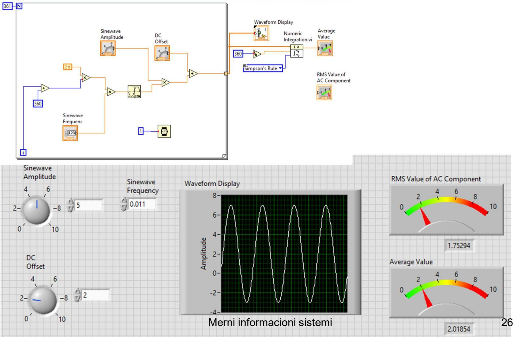
The RMS value of the AC component of the signal
