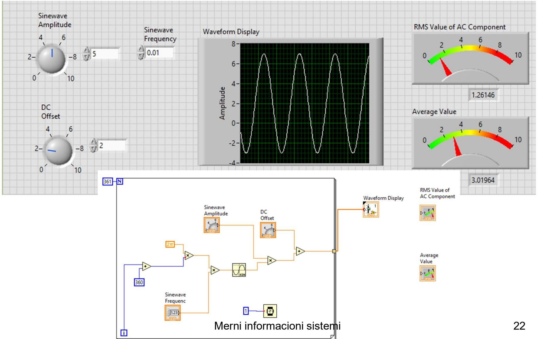
The signal needs to be integrated over one cycle
