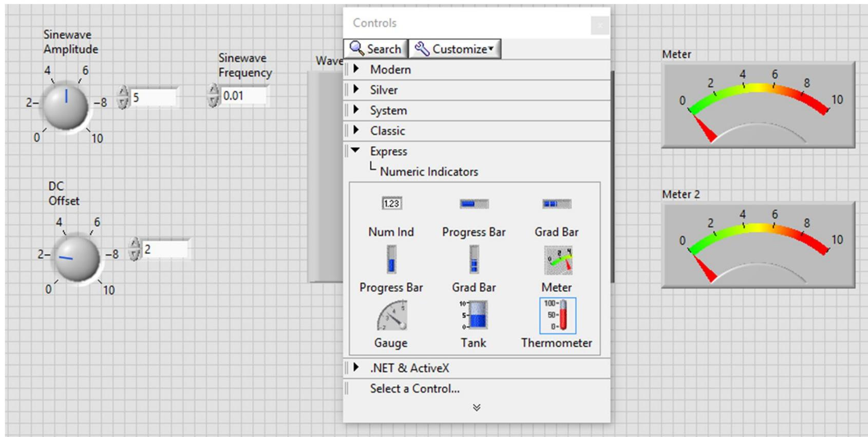
Right-click on each meter and use the Visible Items>Digital Display command to add the digital display
