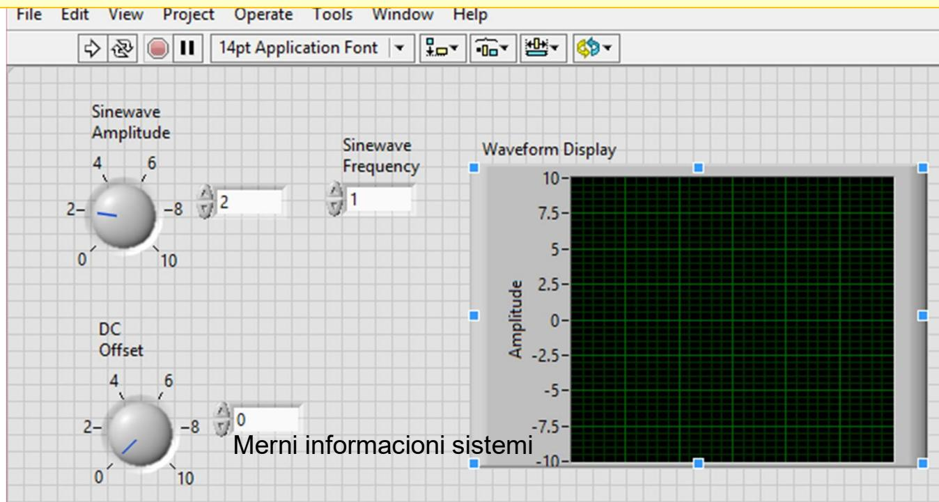
Use the Window>Show Block Diagram command to switch to the block diagram window
