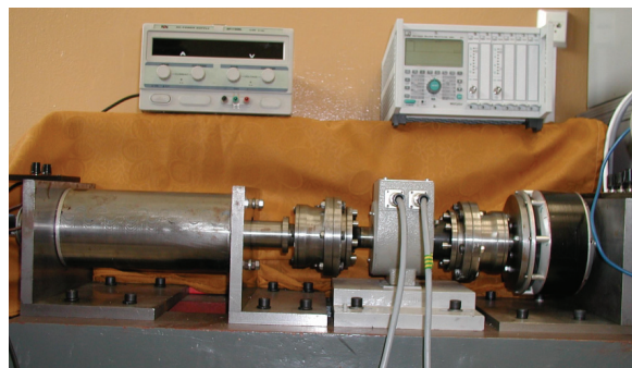
Fig. 15. General view of the measurement set for investigations of the brushless direct current motor
