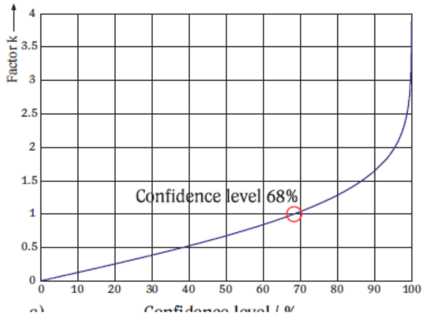
Fig. 5-27 Coverage factor k as a function of confidence level a) confidence level 0% to 100%, b) confidence level 90% to 100% (zoomed)
