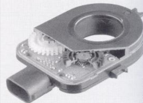
3 LWS4 AMR steering-angle sensor for mounting on the end of the steering axle
