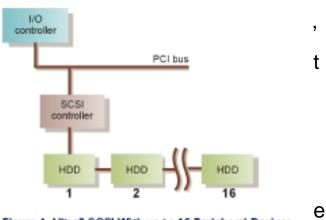
SCSI subsystem. To this end, the <u>SPI-3 standa</u>. Figure 4. Ultra2 SCSI with up to 16 Peripheral Devices overhead required for arbitration. This feature is called *quick arbitration and selection* or *QAS*. You may also see it called by the name it carried during development, *quick arbitration and select*; IBM calls it *quick arbitration select* and Adaptec, simply *quick arbitrate*. These are all different names for the same feature.
