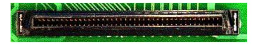
A female 80-pin SCA connector. This is the connector that would be found on a backplane designed for SCA SCSI
