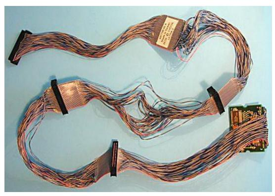
An internal, 68-wire, 5-connector LVD cable. Note the distinctive "loose" twisted pair wiring between the connectors. The circuit board at bottom right is an integrated LVD/SE <u>terminator</u>. (Incidentally, one of the connectors is hidden behind the terminator and hard to see.)
