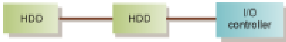
Figure 5. ATA Configuration With Two Peripheral Devices
