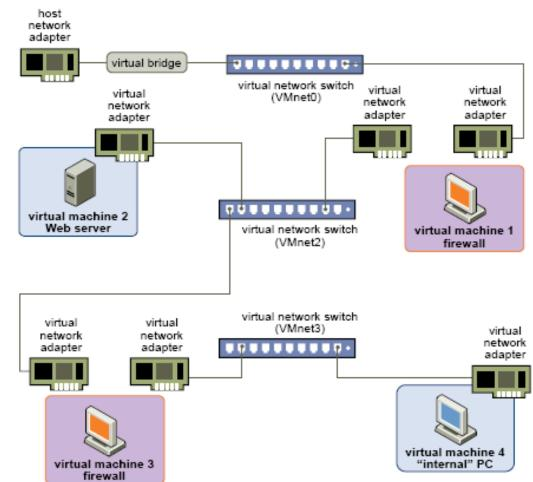
Figure 5-4. Custom Configuration with Two Firewalls
