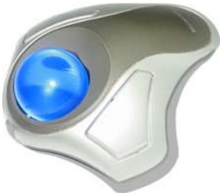
Used as an alternative to a mouse. To operate it the user rotates the ball which moves the pointer on screen. They are particularly easy to use for those with limited movement in their hands and are often used in Computer Aided Design (CAD) for their increased precision over a mouse.
