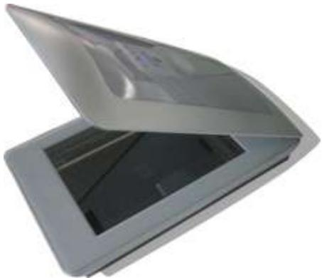
A scanner can be used to digitise images. They're similar to a photocopier but they make a *digital* copy instead of a physical copy. They can also be used with optical character recognition (OCR) software to scan in text that is then editable.
