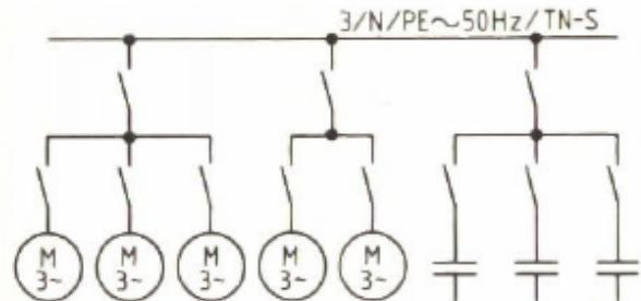
CENTRALNA KOMPENZACIJA UKUPNE REAKTIVNE SNAGE POTROŠAČKOG POSTROJENJA POMOĆU REGULACIONE KONDENZATORSKE JEDINICE
