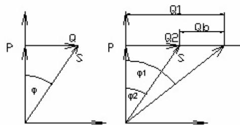
$$S^2 = P^2 + Q^2 \quad \cos \varphi = \frac{P}{S}, \quad \operatorname{tg} \varphi = \frac{Q}{P}$$
