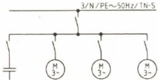
POTROŠAČI REAKTIVNE SNAGE SA JEDNOM PARALELNO SPOJENOM KONDENZATORSKOM JEDINICOM
